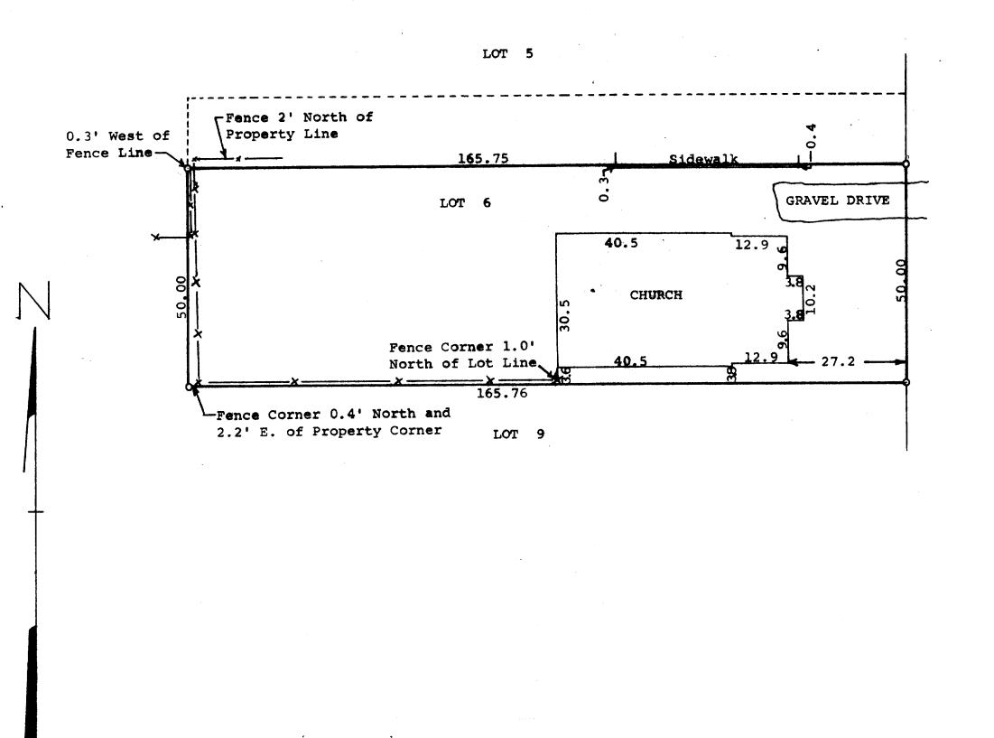
Scale - 1" = 20o = Iron Pipe Set o = Iron Pipe Found x---x= Fence Line
